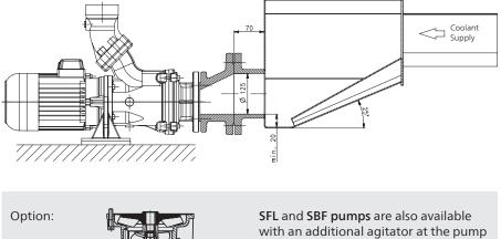
SFL and SBF pumps are also available with an additional agitator at the pump suction. The agitator can either be supplied directly with the pump assembly or is available as a separate component for installation in the field at a later date. SBF pumps are comparable to SFL pumps from a technical standpoint. These pumps can be mounted directly to the machine and are available upon request with upgraded materials of construction which allow for unlimited dry-running (double mechanical seal).
