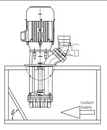
The SFL pump series represents an innovative lift pump concept which has found many pumpback applications world wide. The SFL pumps series can be customized through various options and upgrades.
