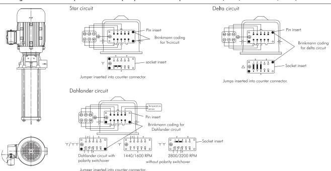
Pin assignment for HAN 10-pin connector for pumps with motors up to 7.5/8.6 kW (400 V, 50 Hz / 460 V, 60 Hz)
