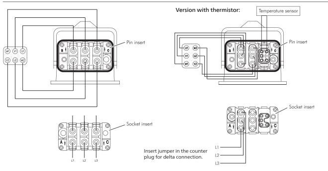
Positions for motor connection plug – View onto terminal board
